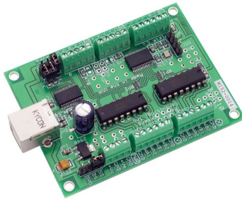
Figure 6.3 Stepper motor control board.
