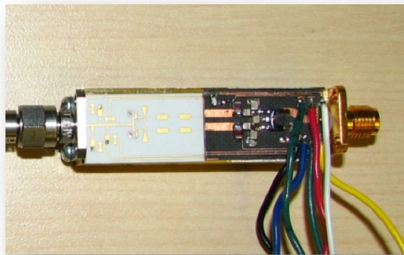
Figure 3.33 Photograph of the proposed 35 GHz self-oscillating mixer.
