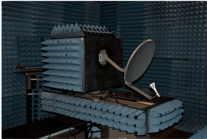
Figure 4.2 Reflector antenna measurement.
