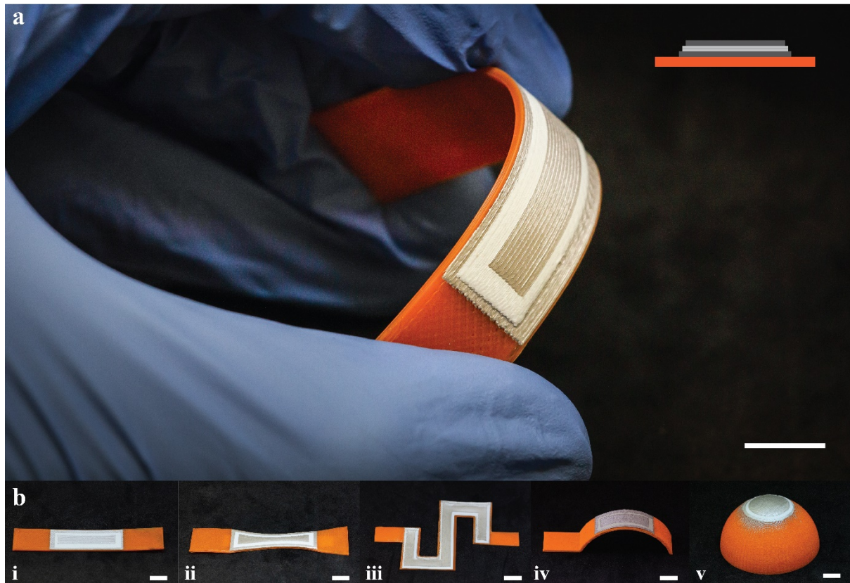
Figure 4. 3D printed flexible piezoelectric devices for monitoring or energy harvesting (scale bar = 10 mm): a Optical image of a flexible piezoelectric energy harvester under bending deformation; inset at the top right shows the schematic of the piezoelectric device with a PLA substrate (orange color) covered with conductive electrodes in grey color and piezoelectric layer in white color, b Piezoelectric energy harvesting demonstrators fabricated by multi-material multi-process additive manufacturing: (i) Straight beam (SB), (ii) variable cross-section beam (VSB), (iii) s-shape beam (SSB), (iv) arc-beam (AB), and (v) semi-spherical shell (SSS).
