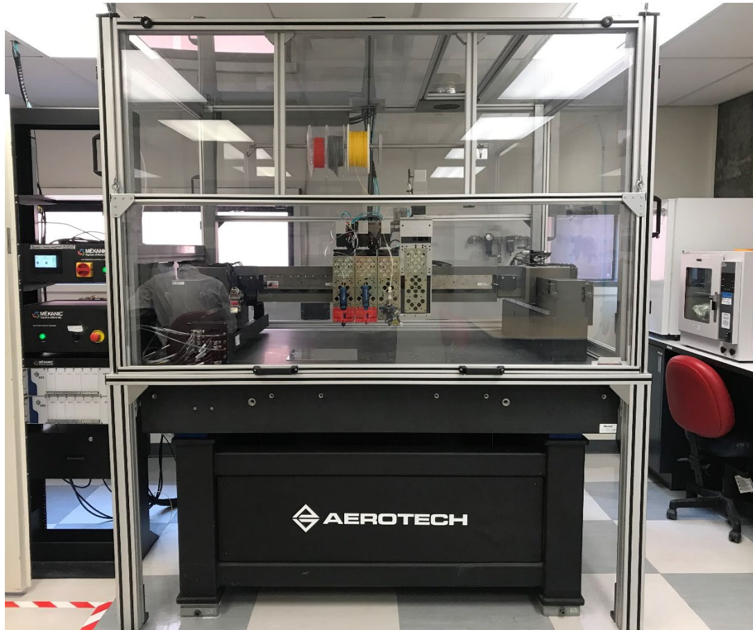
Figure S1. A photograph of Aerotech (ABG10000 model, Aerotech Inc., USA) gantry motion control system. The print bed sits on the x-y motion stage while all printing heads are mounted on the z-direction stages. The machine has a build area of 0.4m x 0.4m , with local accuracy, repeatability, and maximum velocity \pm 2 \mu\text{m} , \pm 0.3 \mu\text{m} , and 120 mm/s, respectively. Each z-axis printhead has 0.15 m of vertical travel, with accuracy, repeatability, and maximum velocity of \pm 0.75 \mu\text{m} , \pm 0.3 \mu\text{m} , and 50 mm/s, respectively.
