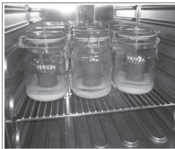
Figure 1. Experimental apparatus for the sorption isotherms measurement.
