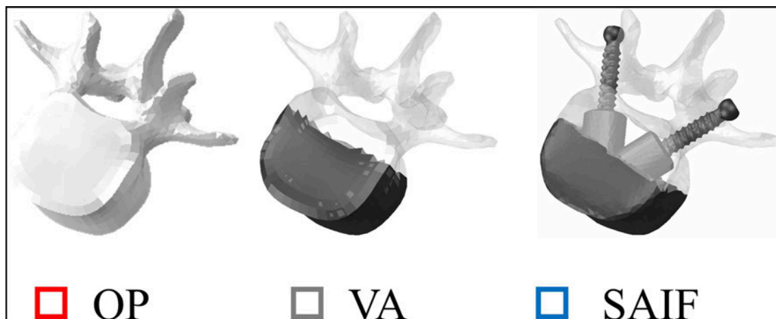
FIGURE 2 | Representation of L3 vertebrae in all simulated conditions. From left to right: osteoporotic vertebra (OP) taken as a reference condition, vertebral augmentation (VA) and the new Stent-Screw Assisted Internal Fixation (SAIF). Bone is highlighted in shaded white, while screws and bone cement are in dark grey.
