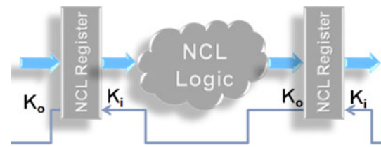
Fig. 6 Representation of the NCL pipeline
