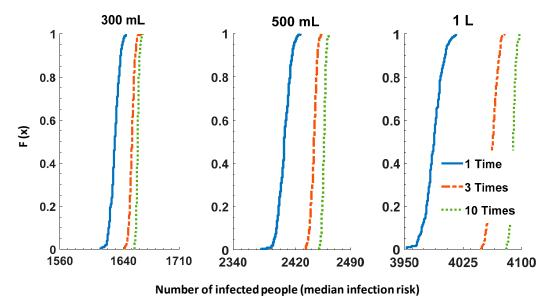
**Figure 5.** Impact of consumption volumes and number of glasses per day on the number of infected people corresponding to median infection risk over a four day-period; *Cryptosporidium* concentration = 560 oocysts/L; the x-axis scale is the same between the plots (150 people).
