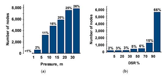
**Figure 2.** Distribution of: (a) nodal pressures for the whole network (30,077 nodes); and (b) demand satisfaction ratios (DSRs) for nodes under pressure-deficient conditions (8578 nodes), excluding the nodes with zero demand.
