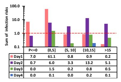
**Figure 11.** Number of infected people for different pressure (P) ranges (based on the pressure values under PDCs) on Days 1–4; Infection risks corresponding to the consumption event with F(x) = 1 (Figure 8) are illustrated. The event starts at 18:30 on Day 1 for a duration of 1 h. Daily patterns in the hydraulic model.
