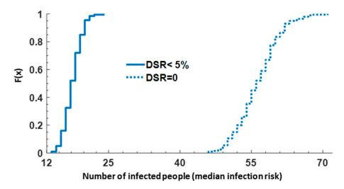
**Figure 10.** Probability distributions of the number of infected people during the first day of simulation when people with a DSR null and less than 5% do not drink water from tap; 200 Monte Carlo simulations for each scenario;  $C_{out} = 560$  oocysts/L with 1 h of PDCs with daily consumption patterns.
