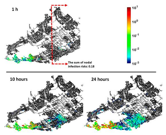
**Figure 7.** Spatial distribution of nodal risks for three durations of PDCs: 1, 10, and 24 h; *Cryptosporidium* concentration in sewage = 560 oocysts/L; nodes with an infection risk below  $1 \times 10^{-3}$  are drawn in black; infection risks corresponding to consumption events with F(x) = 1 (Figure 6) are illustrated.
