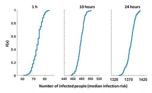
**Figure 6.** Comparing the probability distribution of the number of infected people over a four-day period for 200 Monte Carlo simulations for each duration of PDCs: 1, 10, and 24 h; *Cryptosporidium* concentration in sewage = 560 oocysts/L.
