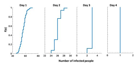
**Figure 8.** Number of infected people corresponding to median infection risk for Days 1–4 for the scenario of 1 h of PDCs with daily consumption patterns;  $C_{out} = 560$  oocysts/L; 200 Monte Carlo simulations (consumption events) every day.
