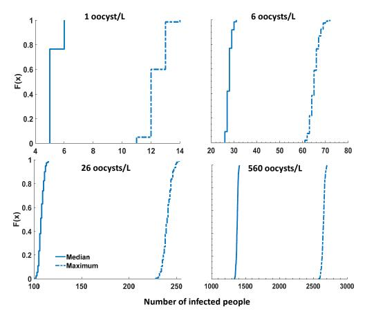
**Figure 4.** Number of infected people corresponding to median and maximum infection risks resulting from a 24-h depressurization; 200 Monte Carlo simulations (consumption events) for each *Cryptosporidium* concentration: 1, 6, 26, and 560 oocysts/L; number of infected people corresponds to the cumulative dose over four days of observation; F(x): probability that the median/maximum number of infected people will be less than or equal to x.
