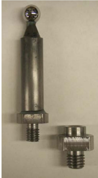
Figure 3.1 Artefact module sub-assembly with an adapter.
