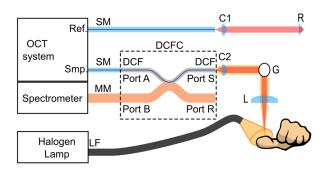
**Fig. 1** Optical setup: Ref, reference arm port; Smp, sample arm port; SM, single-mode fiber; MM, multimode fiber; DCF, double-clad fiber; DCFC, double-clad fiber coupler; C1 and C2, collimation lenses; G, dual-axis galvanometers; L, focalization lens; R, retroreflector prism; LF, light guide fiber.
