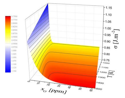
**Figure 2.** Predicted, via Eq. 8, surface tension of liquid aluminium as a function of temperature and oxygen content. Parameters for Eq. 8:  $\Gamma_O^{sat.} = 1.65 \times 10^{-5} \text{ mol.m}^{-2}$ ,  $\sigma_O^{sat.} = 0.86 \text{ J.m}^{-2}$  and  $x_O^{sat.}$  is a function of temperature calculated by Eq. 13.
