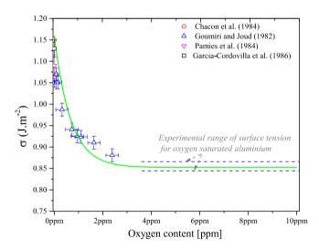
**Figure 3.** Predicted surface tension of liquid aluminium as a function of oxygen content at melting temperature (933 K) (solid line) in comparison with experimental data at the same temperature (open symbols). References: Chacon *et al.*<sup>28</sup>, Goumiri and Joud<sup>2</sup>, Pamies *et al.*<sup>29</sup>, Garcia-Cordovilla *et al.*<sup>3</sup>. The two dash lines represent the standard deviation of the mean experimental surface tension of oxygen saturated aluminium<sup>1,10,26,27</sup>.
