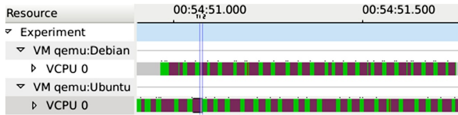
Figure 12 vCPU0 of Debian and vCPU1 of Ubuntu are taking turns in execution, which indicates competition over a shared resource. The figure also shows some timeframes in which both vCPUs are preempted, most probably by a different thread on the host system.
