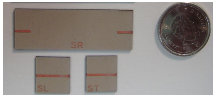
Fig. 3.8 TRL calibration kit
