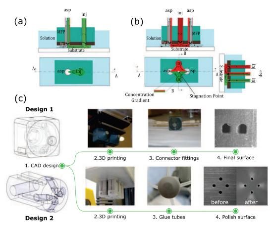
**Figure 1.** 3D Printed MFPs. (a) MD configuration of the MFP and its operating principles. (b) MQ configuration of the MFP and its operating principles. (c) 3D printing fabrication steps for both designs of the MFP.
