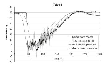
**Figure 2.** Comparison of pressures recorded at one distribution system site with pressures modelled with typical wave speeds and with a reduced wave velocity in cast-iron pipes (four pressure values per second were measured by the pressure recorders but only the minimum and maximum pressures over 15 s intervals were saved ( $\triangle$  and  $\triangle$ ).
