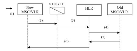
Fig. 1. Updating procedure according to IS-41 standard.
