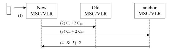
Fig. 4. Updating procedure for an intra-ILD move.
