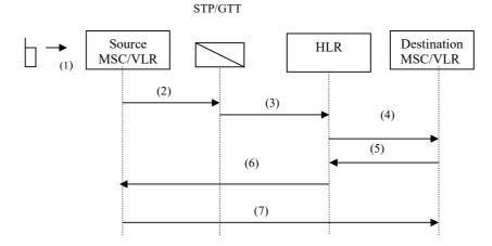
Fig. 2. Location search procedure according to IS-41 standard.
