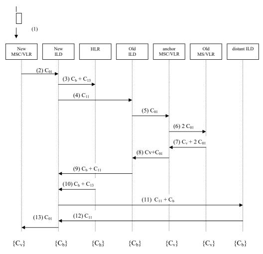
Fig. 5. Updating procedure for an inter-ILD move.
