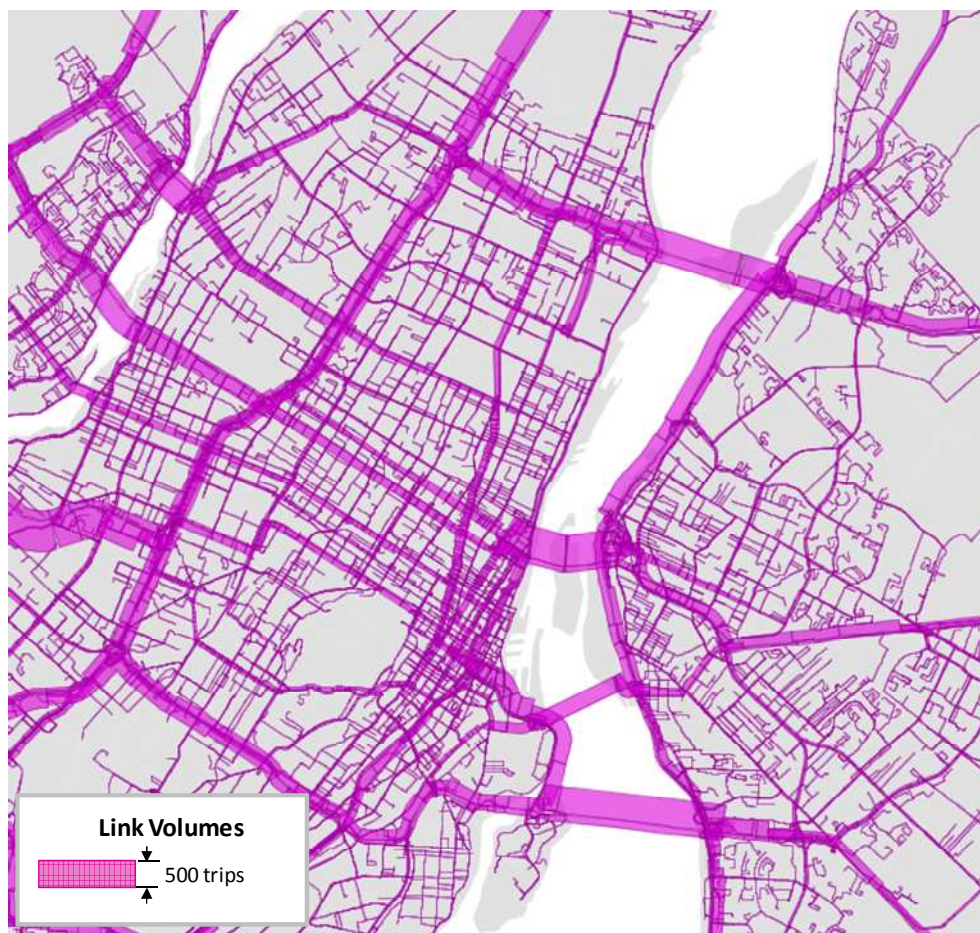
Figure 2.37: Flow map produced using a totally disaggregate assignment of bridge traffic for the a.m. peak period
