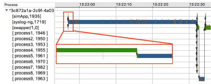
Fig. 17. Active path of the application simulator. Some sensitive information like process's names were hidden, due to privacy concerns.
