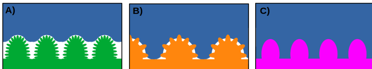
Figure 3.1 Illustration of (A) Cassie-Baxter wetting state, leading to the lotus effect ; (B) Cassie impregnated wetting state, leading to the petal effect ; (C) Wenzel wetting state is the fully impregnated Cassie-Baxter wetting state. Blue represents water, white represents air pockets trapped between the surface and the liquid, other colors are for solid materials (For interpretation of the references to colour in this figure legend, the reader is referred to the web version of this article).
