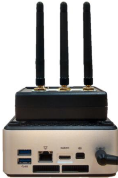
Figure 4. 6 Intel NUC mini PC, equipped with NIC 5300, presented in [30].
