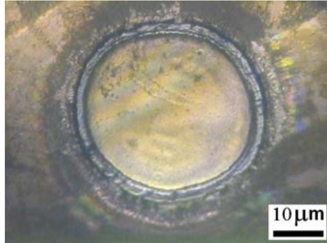
Figure 2.30: Incomplete hole with 30 \mu\text{m} diameter and 3 \mu\text{m} depth.
