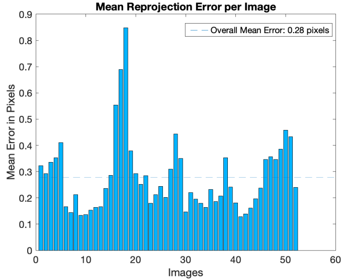
Figure 5.5 Mean reprojection error of the acquired images of Zhang's method
