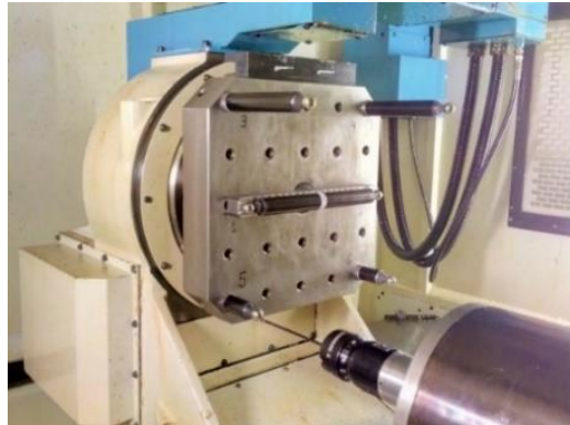
Figure 4-9. The laboratory a five-axis machine tool undergoing a SAMBA test
