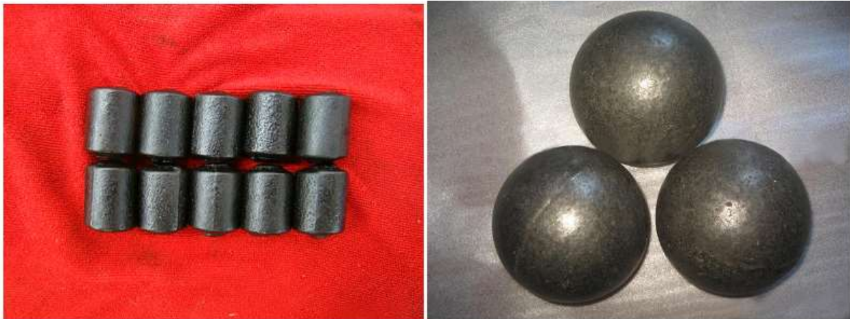
Figure 2.6 Commercial grinding media in ball milling, Cylpebs versus balls
