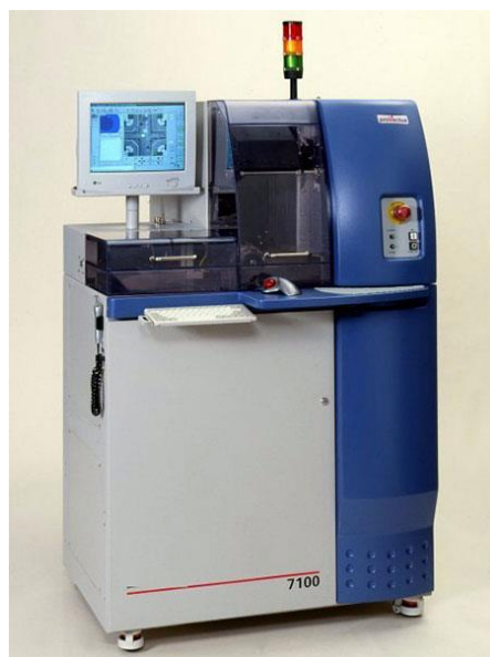
Figure 3.6 ADT 7100 dicing machine (Image courtesy: University of Michigan)
