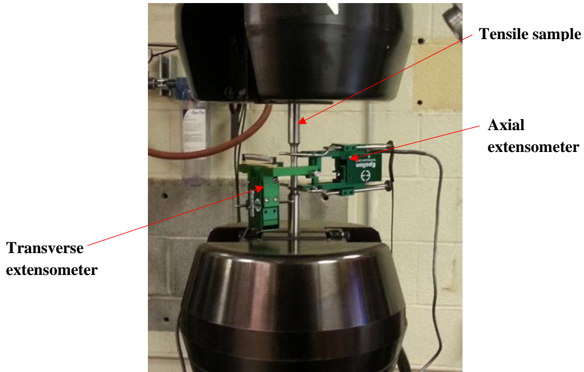
Figure 4.2 Tensile test setup for cylindrical 300M steel samples with axial and transverse extensometers
