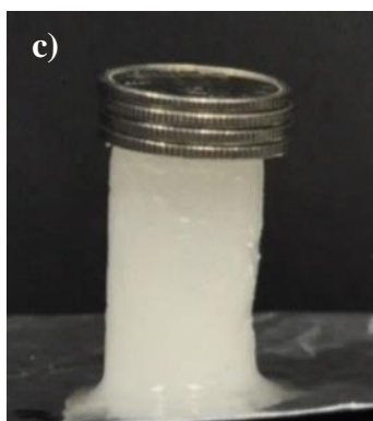
Figure 5.6 a) Normalized height ( h(t)/h_0 ) as a function of time t and applied stress on molded concentrated emulsions ( \phi_o = 0.8 ) comprising 4% SP or SP-SA particles, at pH 3.0 and 7.0; b-c) visual aspect of the solid-like behavior of molded Pickering emulsions comprising 4% SP-SA particles, compared to a concentrated emulsion prepared with pristine SP displaying no yield stress, at pH 3.0;
