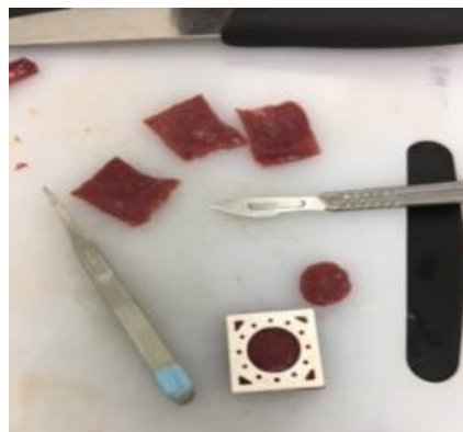
Figure 3.2 Samples being prepared before being placed in the Rheometer
