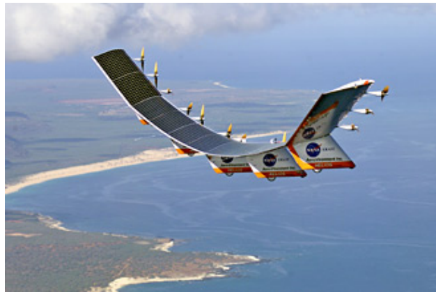
Figure 1.4 NASA Helios, a solar powered prototype showing large deflection during flight [4]
