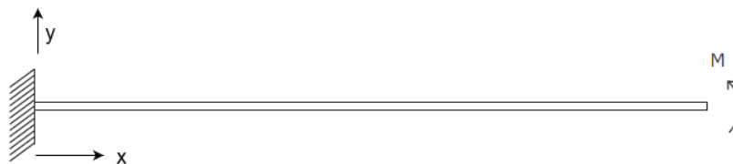
Figure 4.2 Beam with moment applied at free end
