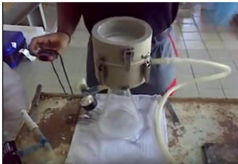
Figure 8.3 : Buchner test kit from Outotec Larox ®37
