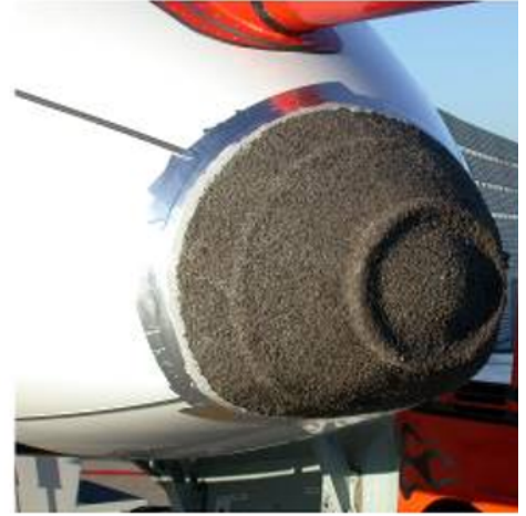
(b) Machined ice shape on the nose
