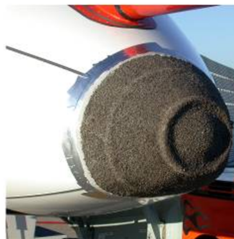
(b) Machined ice shape on the nose
