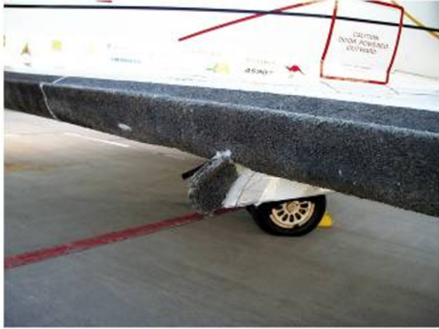
(a) Machined ice shape on wing leading edge
