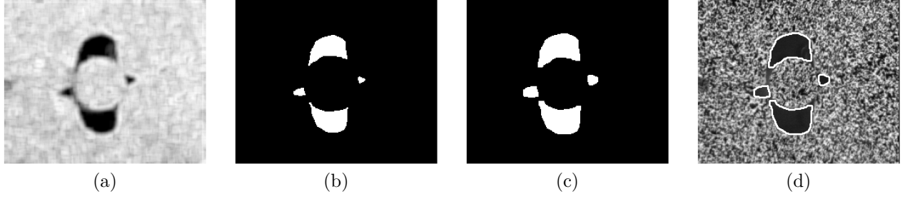
Figure 6.6 Crack extraction using texture features in the original camera images for the PTFE / epoxy specimen with \bar{\sigma} = 20.2 MPa and \bar{\epsilon} = 6.66 %. ((a)) Local entropy of the camera image. ((b)) Local entropy after thresholding into a binary image. ((c)) Final image after compensating for the local entropy subset size. ((d)) Contour of the final image overlayed over the original camera image. The image based method appears to underestimate the crack area.
