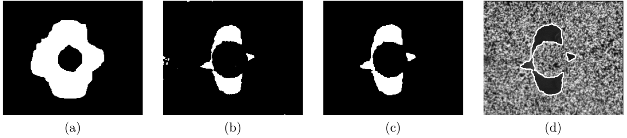
Figure 6.7 Crack extraction using the hybrid method for the PTFE / epoxy specimen with \bar{\sigma} = 20.2 MPa and \bar{\epsilon} = 6.66 %. ((a)) DIC-based crack estimate after a round of dilations. ((b)) Image-based crack estimate using a smaller subset size. Note the false-positive regions produced by imperfections in the speckle pattern. ((c)) Final image after combining the DIC- and image-based estimates. ((d)) Contour of the final result overlayed over the original camera image. The hybrid method appears to produce an accurate crack area estimate.
