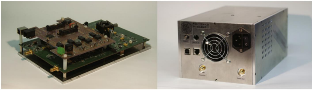
Figure 2.28. Fast-gated module [88] consisting of two boards (left) and its housing (right)
