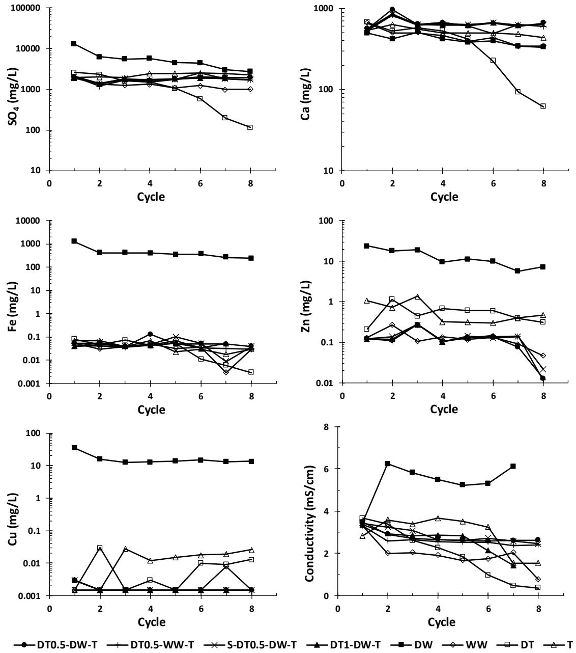
Figure 4.5 : Metal concentrations (mg/L) and electrical conductivity (mS/cm) measured in the column leachates.
