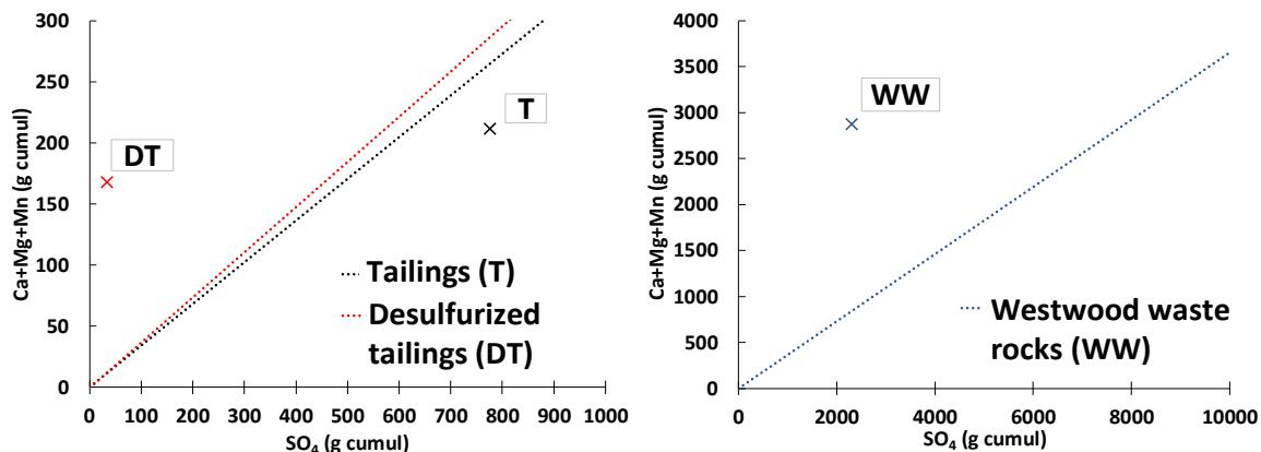
Figure 4.6 : Extrapolation of the oxidation neutralization curve and initial composition of tailings
