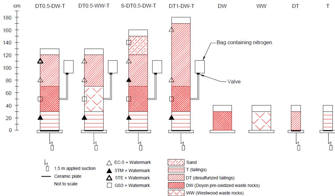
Figure 4.1 : Configuration and instrumentation of the column tests.
