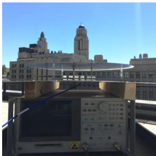
Figure 3-45: Outdoor testing of the dual-band antenna.
