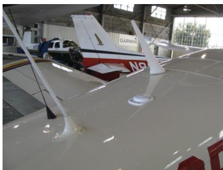
Figure 1-2: Blade and whip antenna placed on an aircraft [5].
