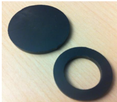
Figure 5-5: Samples for testing the dielectric and magnetic properties of TTZ500.
