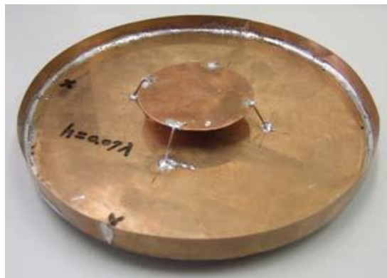
Figure 2-10: Fabricated prototype of top-loaded monopole antenna © 2009 IEEE [39].
