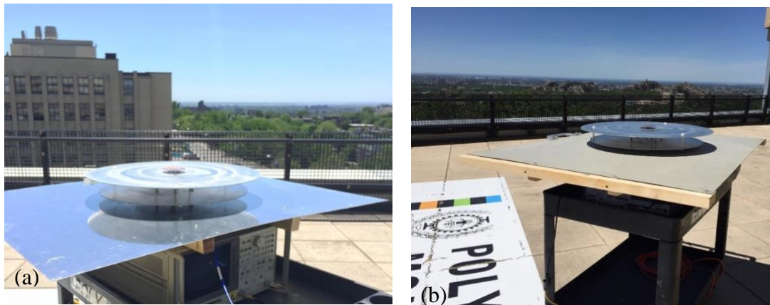
Figure 3-46 : Outdoor measurements (a) Aluminium ground connected to the antenna, (b) Composite ground connected to the antenna.
