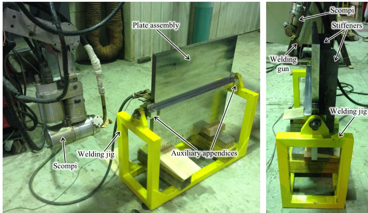
Figure 3.2: Plate assembly with auxiliary appendices and stiffeners installed on the welding jig. A Scompi robotic welding machine [130] is located next to the welding jig
