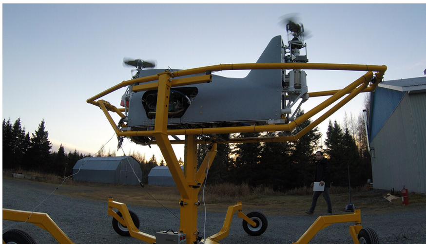
Figure 3.11 Banc de test 4DOF du drone, © 2018 LAFLAMME AERO INC.
