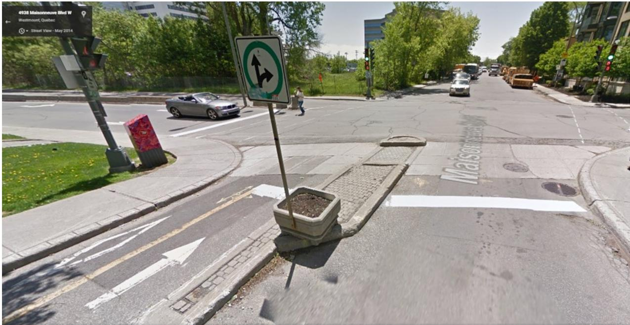
Figure C. 1 End of cycle track where cyclists wishing to continue through the intersection must move to the right hand side of the lane with cars moving in the opposite direction (Google images, Montréal: Maisonnette and St. Catherine)
