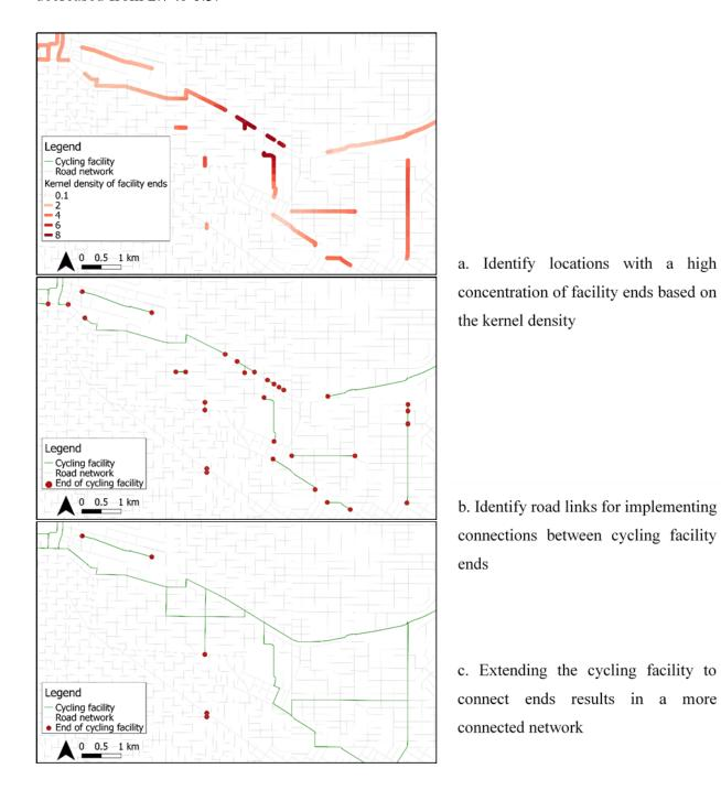
Figure 4-6 Improving the connectivity of the cycling network by connecting the cycling facility ends
