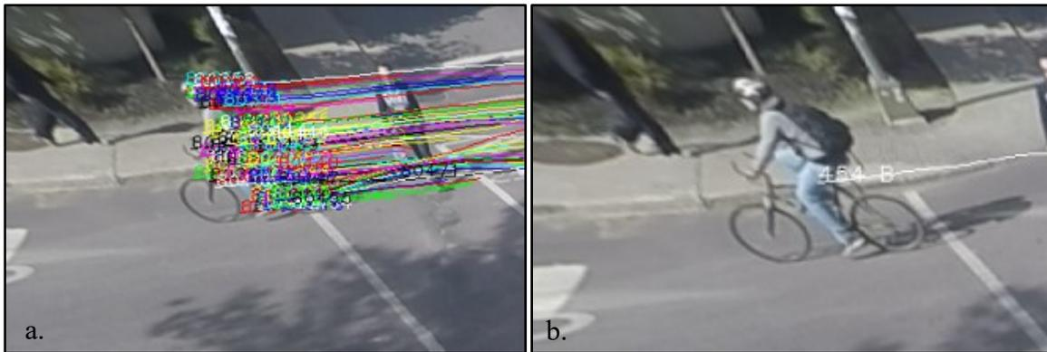
Figure 3-11 a. Tracked features over a cyclist, and b. grouped cyclist features
