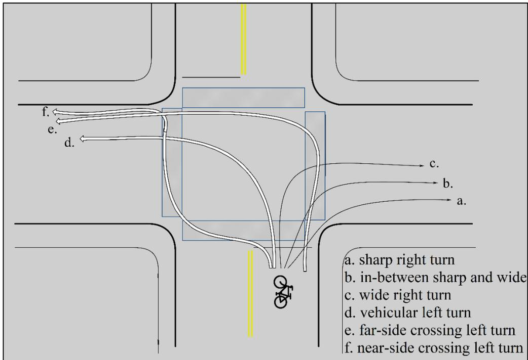
Figure 7-1 Some possible right and left turning movements
