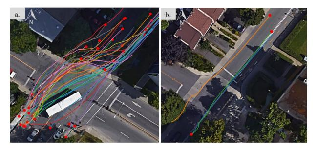
Figure 7-5 Cyclist motion patterns under study at the a. site with discontinuity, and b. the control site (origins marked with a red circle)
