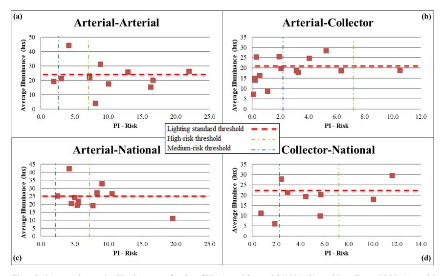
Figure B. 5 Average intersection illuminance as a function of PI: (a) arterial – arterial (14 %), (b) arterial – collector (18 %), (c) arterial – national (14 %), and (d) collector – national (12 %). 42 % of the intersections are not represented in these plots
