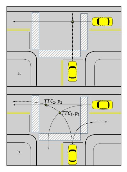
Figure 2-3 a. Traditional motion prediction method assuming constant speed and direction, b. probabilistic motion prediction method using observed motion patterns
