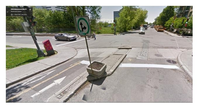
Figure C. 1 End of cycle track where cyclists wishing to continue through the intersection must move to the right hand side of the lane with cars moving in the opposite direction (Google images, Montréal: Maisonneuve and St. Catherine)
