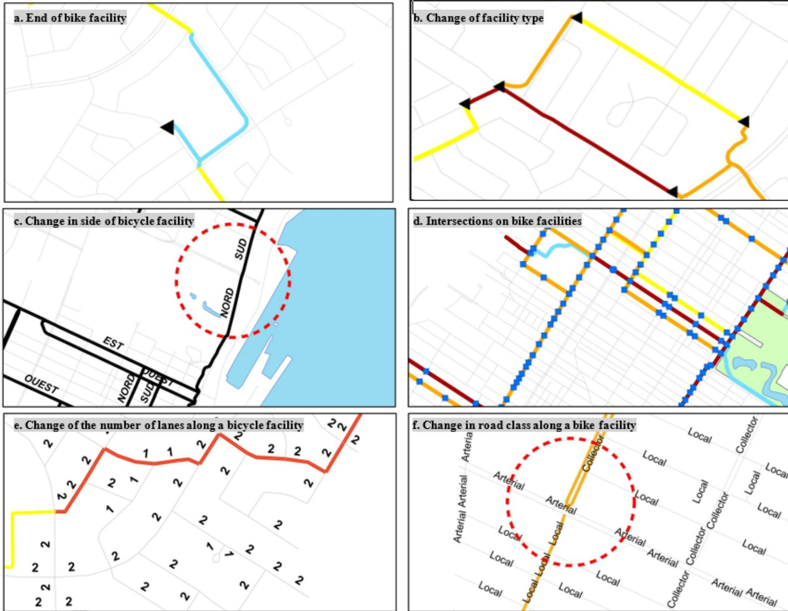
Figure C. 3 Illustration of different bicycle network discontinuity measures
