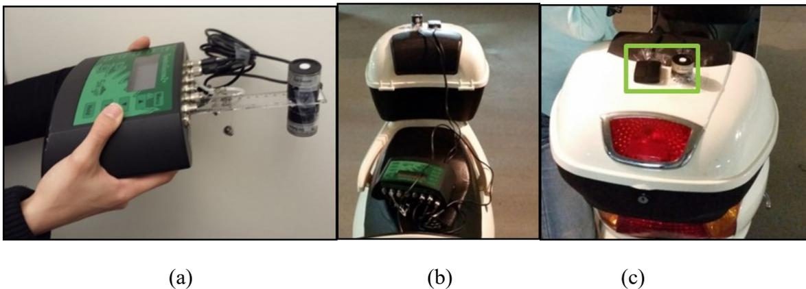
Figure 5-1 a. Data logger and sensor held by the data collector; b. and c. illuminance sensor and GPS mounted on electric scooter
