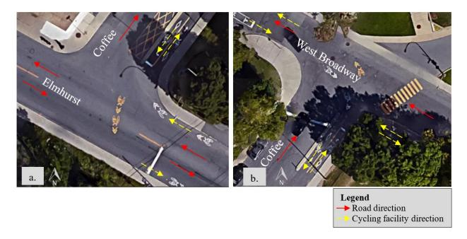
Note: the aerial view of the intersection b. Coffee and West Broadway has the physically separated cycling facility blocked by trees, the yellow arrows indicate the location where the facility exists
