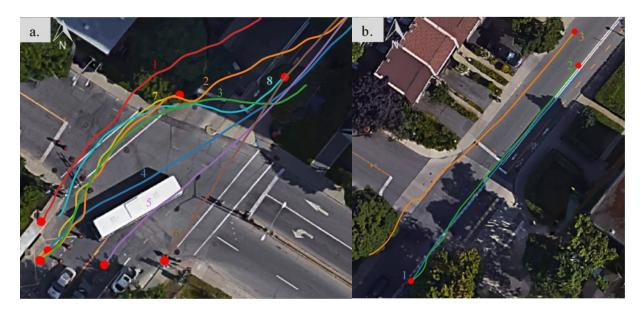
Figure 7-6 Cyclist motion patterns under study with cyclist-vehicle interactions with a collision course at the a. discontinuity location, and b. control site (origins marked with a red circle)
