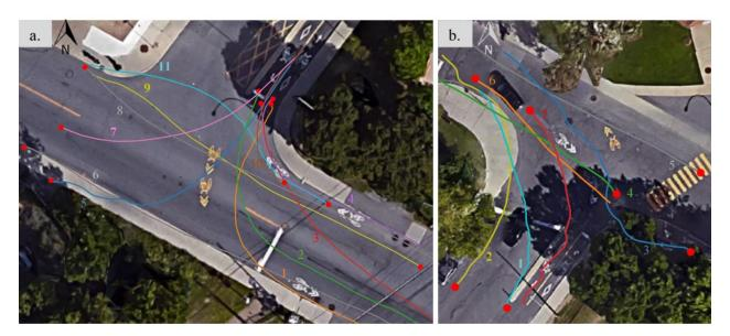
Figure 7-8 Cyclist motion patterns under study at the a. site with discontinuity location, and b. control site (origins marked with a red circle)
