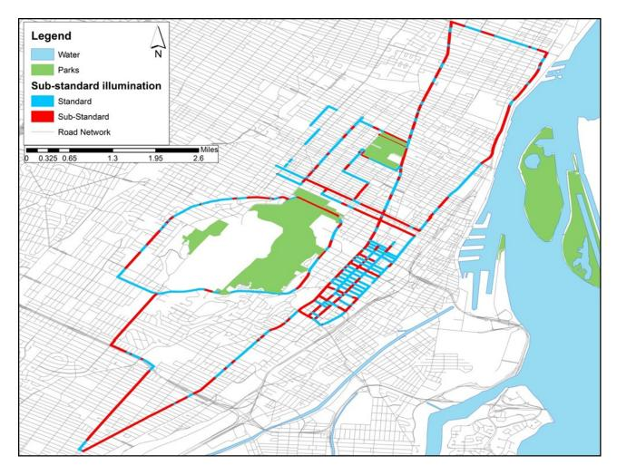
Figure 5-5 Substandard lighting shown in red and standard lighting shown in blue representing the non-uniform lighting of links
