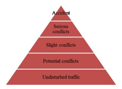
Figure 2-2 Safety pyramid (adapted from (Hyden, 1987))
