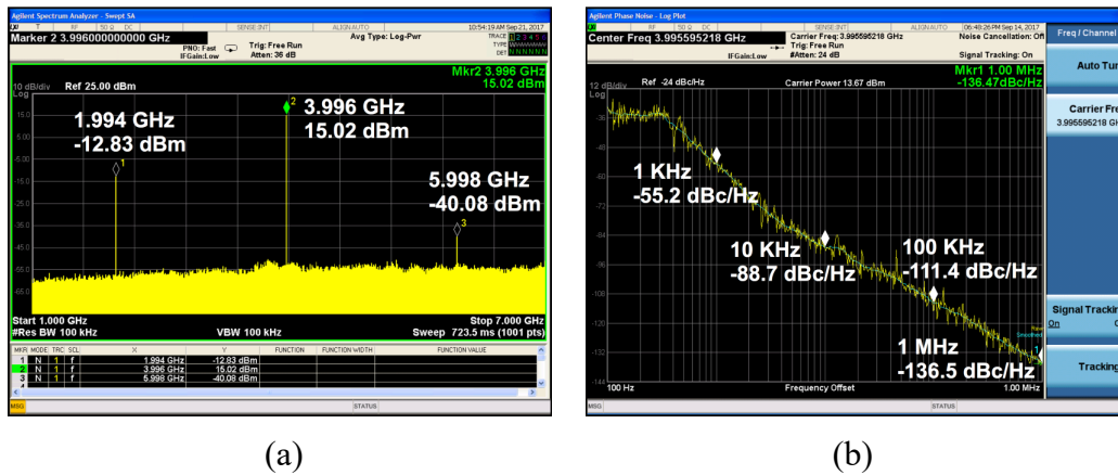
Figure 4.18: Measured results with a 50 \Omega load of (a) spectrum of the first three harmonics, and (b) phase noise of the 2 nd harmonic output.
