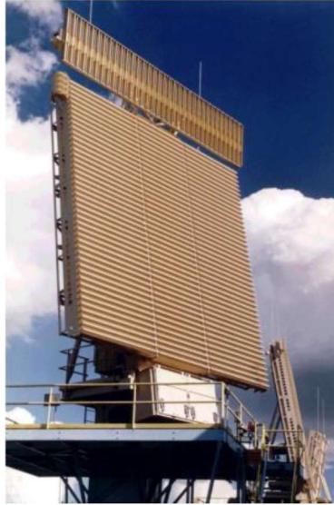
Figure 2.2: AN/FPS-117, 3-dimensional air research radar, Lockheed Martin.
