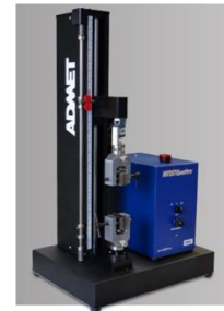
Figure 5.31: ADMET eXpert 7600 UTM series specs. Adopted from [126]
