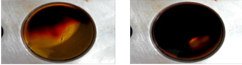
Figure 3.6: Color change representative of the liquid to gel transformation
