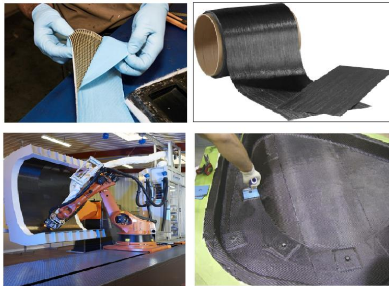
Figure B.6: Prepreg sheet, roll and lay-up [140-143]
