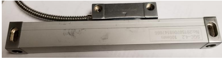
Figure 5.28: Linear optical encoder with 1 \mu\text{m} of resolution
