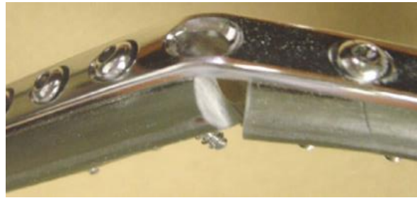
Figure 2.28: Locking plate failure (Ahmad, Nanda et al. 2007)
