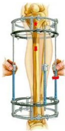
Figure 2.7: Ilizarov ring fixator (Smith&Nephew 2018)
