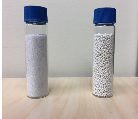
Figure 3-5: Filter bed material: Calcite (left) and Corosex TM (right)
