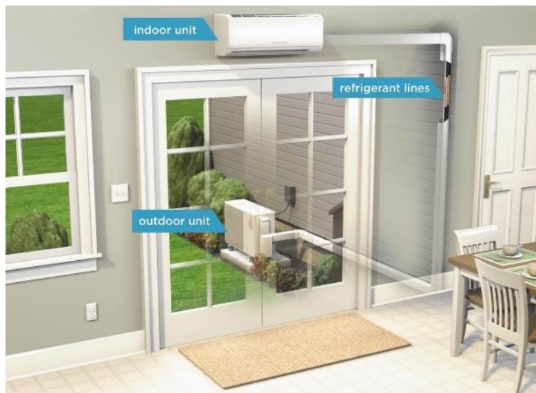
Figure 1-6: Typical mini-split ASHP installation (Energy Star 2018)
