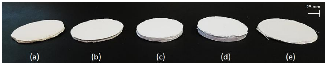
Figure 6-4 : Cakes produced by the filtration device at a pressure of 415 kPa after (a) 1 hour, (b) 2 hours, (c) 4 hours, (d) 6 hours and (e) CMC sample produced at 415 kPa and at V_f = 50\%
