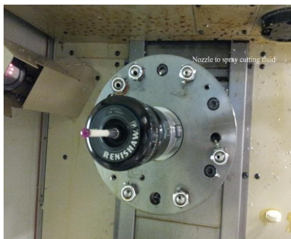
Fig. 2. Spindle with nozzle to spray cutting fluid holding the probe
