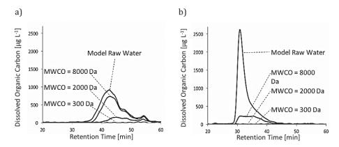
**Figure 2.** Typical size exclusion chromatograms of model raw water and permeate samples: (a) model raw water containing Suwannee River natural organic matter (SRNOM) at 10 mg/L; (b) model raw water containing alginate at 10 mg/L. Dalton values correspond to the molecular weight cut offs (MWCOs) of the different membranes; note that the retention time of the chromatograms is inversely proportional to the log of the molecular weight.
