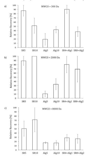
**Figure 4.** Relative recovery during post-clean water filtration (a) MWCO = 300 Da; (b) MWCO = 2000 Da; (c) MWCO = 8000 Da; SR5: SRNOM at 5 mg/L; SR10: SRNOM at 10 mg/L; Alg5: Alginate at 5 mg/L; Alg10: Alginate at 10 mg/L; SR4 + Alg1: SRNOM at 4 mg/L + alginate at 1 mg/L; SR8 + Alg2: SRNOM at 8 mg/L + alginate at 2 mg/L; error bars correspond to observed minimum/maximum values).
