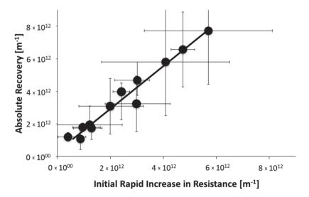
**Figure 5.** Correlation between Absolute Recovery and Initial Rapid Increase in Resistance (model raw waters containing SRNOM and a mixture of SRNOM + alginate; solid line: linear regression,  $R^2 = 0.97$ , slope =  $1.31 \pm 0.35$ , intercept =  $3 \times 10^{11}$ ; p = 0.05; error bars correspond to minimum/maximum values).
