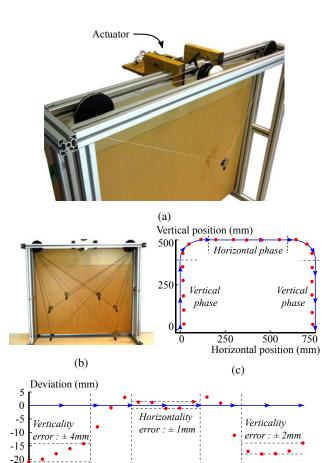
Fig. 7: Experimental results for the trajectory guiding robot. In a), an overall view of the prototype is provided, with a composite photograph of its motion shown in b). Position measurements (in blue), are superimposed on the expected trajectory (in red) in c). In d), the trajectory is unfolded to show the experimental deviations.
