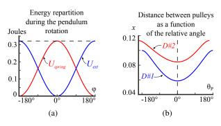
Fig. 8: Static balancing of a pendulum. In a), the constant total energy is shown for  $-\pi < \phi < pi$ . In b), the target distance function is illustrated for both considered designs.
