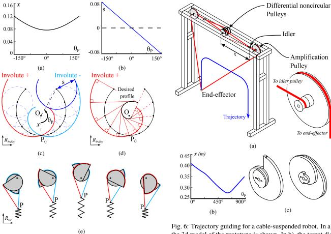
Fig. 5: Proposed synthesis method for the differential case. In a) the target distance is shown, in b) the length of cable transfered from  $l_{F+V}$  to  $l_{F-V}$  is illustrated, in c) the involute curves are drawn, and, in d) the winding pulley shape is obtained from its involute curve. The rotation of the differential pulley system in the external axes system is shown in e).
