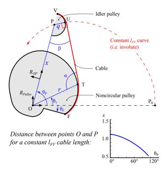
Fig. 1: Geometry of a single noncircular pulley
