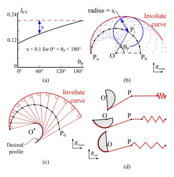
Fig. 2: Illustration of the proposed noncircular pulley synthesis method. In a) the target function  $g(\theta_P, x, l_{FV}) = 0$  is shown, in b) the involute curve is drawn, and, in c) the pulley shape is obtained from the latter curve. The rotation of the noncircular pulley in the external axes system is shown in d).
