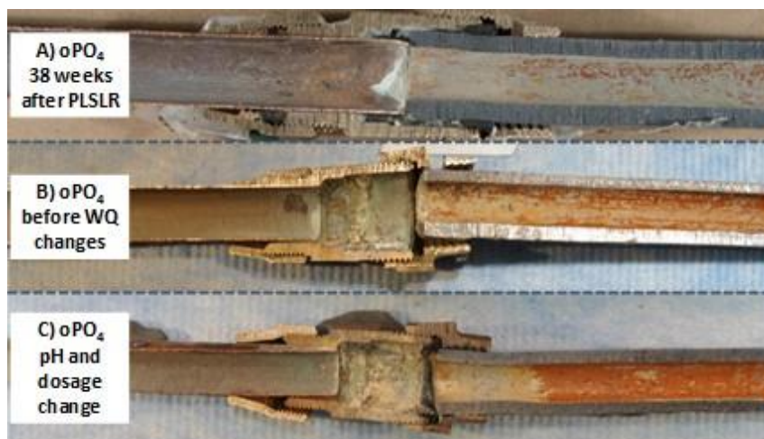
Figure 8.13 Interior of an orthoP treated partial LSL (A) shortly after PLSLR simulation, (B) before changes in water quality and (C) after an increased in orthoP (1 vs 1.5 mg P/L).
