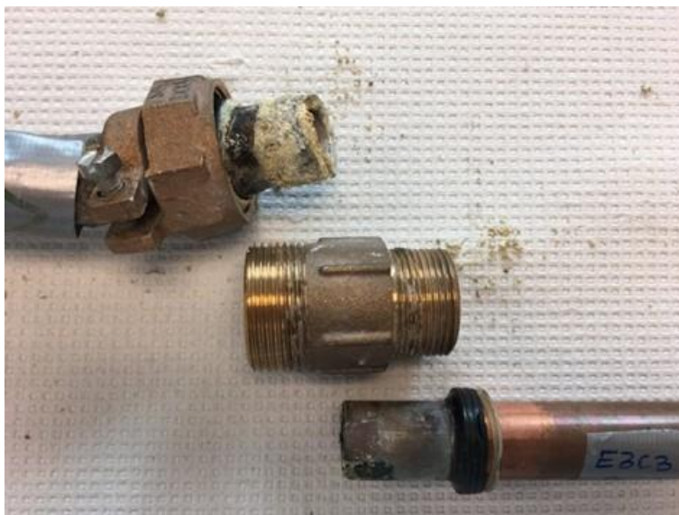
Figure 5.4 Example of a Pb-Cu pipe under the control condition showing external corrosion of the Pb and Cu pipes.
