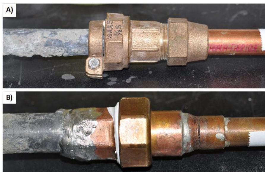
Figure 3.3 An example of a lead service line connected to a copper pipe using (A) a red brass compression fitting and (B) a soldered fitting.
