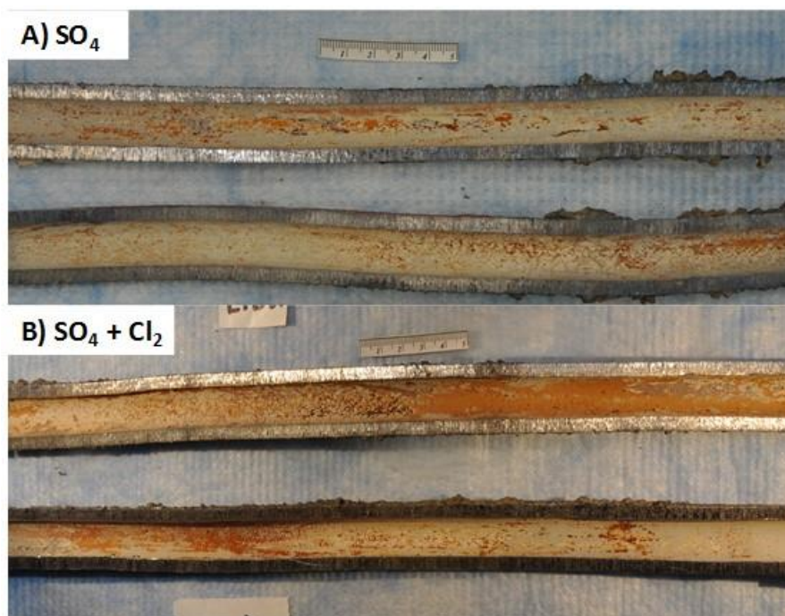
Figure 8.5 Full LSL treated with the addition of sulfate (A) and the combination of sulfate and chlorine (B).
