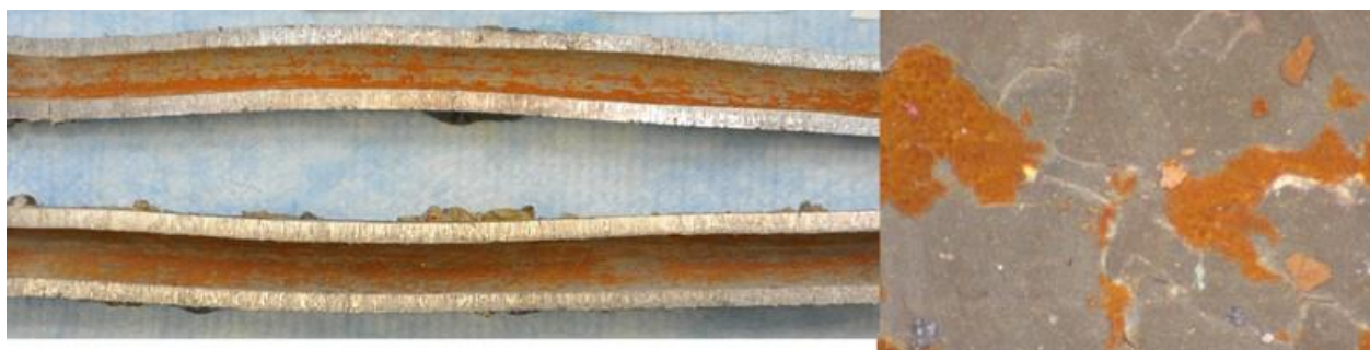
Figure 8.1 Example of surface layers with islands of red deposits (pipe treated with orthoP).
