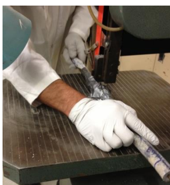
Figure 3.4 Example of a full LSL being prepared for scale analysis.
