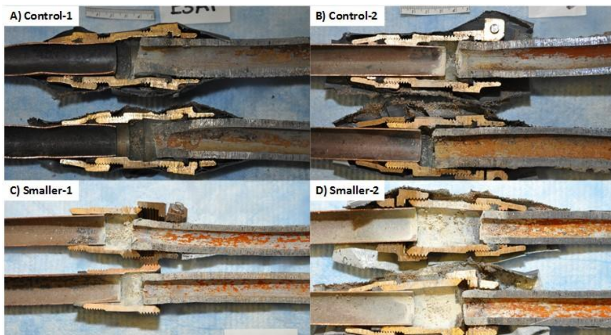
Figure 8.10 Partial LSL of the control condition (A) without visual changes in scale composition at the galvanic zone and (B) with visual changes and for two duplicate pipes of the smaller diameter (C and D).
