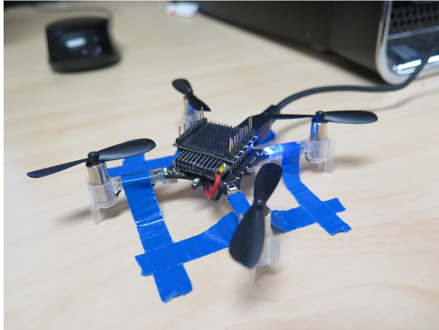
Figure 3.4 Test Bench for Accelerometer Variance Data
