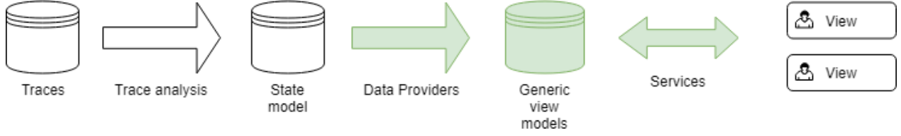
Figure 4.3 Proposed trace analysis server architecture
