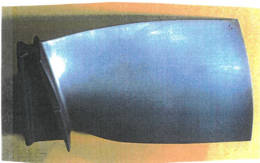
Figure 2.10 Turbine blade used for evaluating the method.
